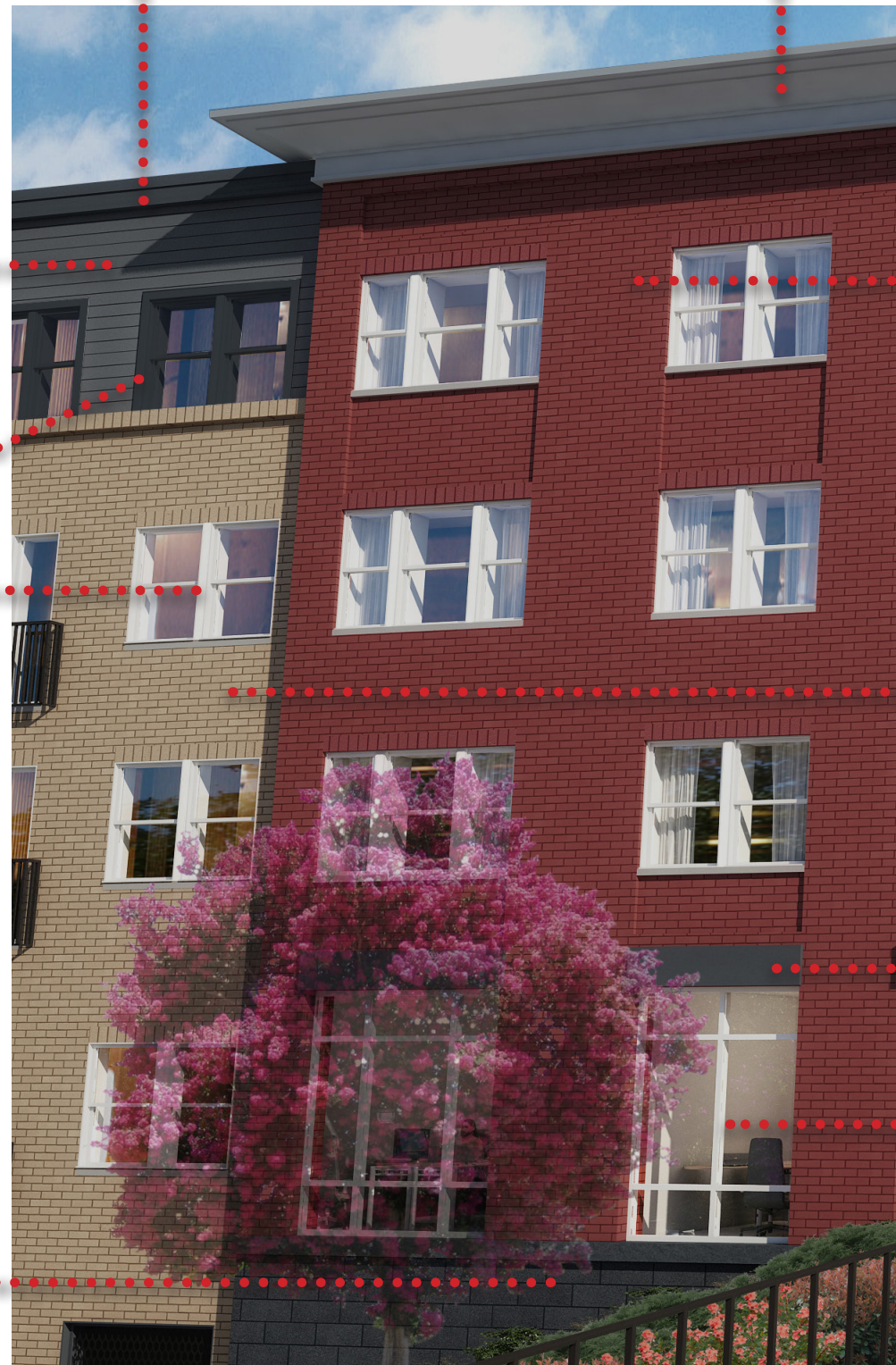
MI WINDOWS VINYL 1-OVER 1 SINGLE HUNG WINDOWS. WHITE AT ALL BRICK; BLACK AT ALL OTHER CONDITIONS
